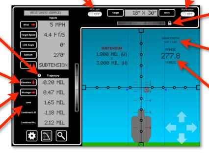
Target Size Locked (Locked when real shaped target selected)
